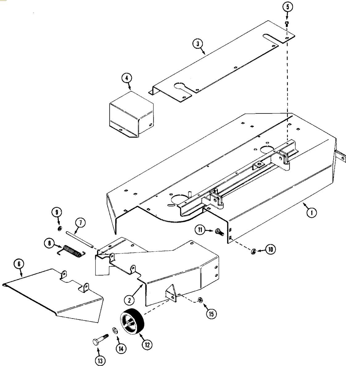
**RM42G ROTARY MOWER****INDEX****DECK AND CHUTE**
