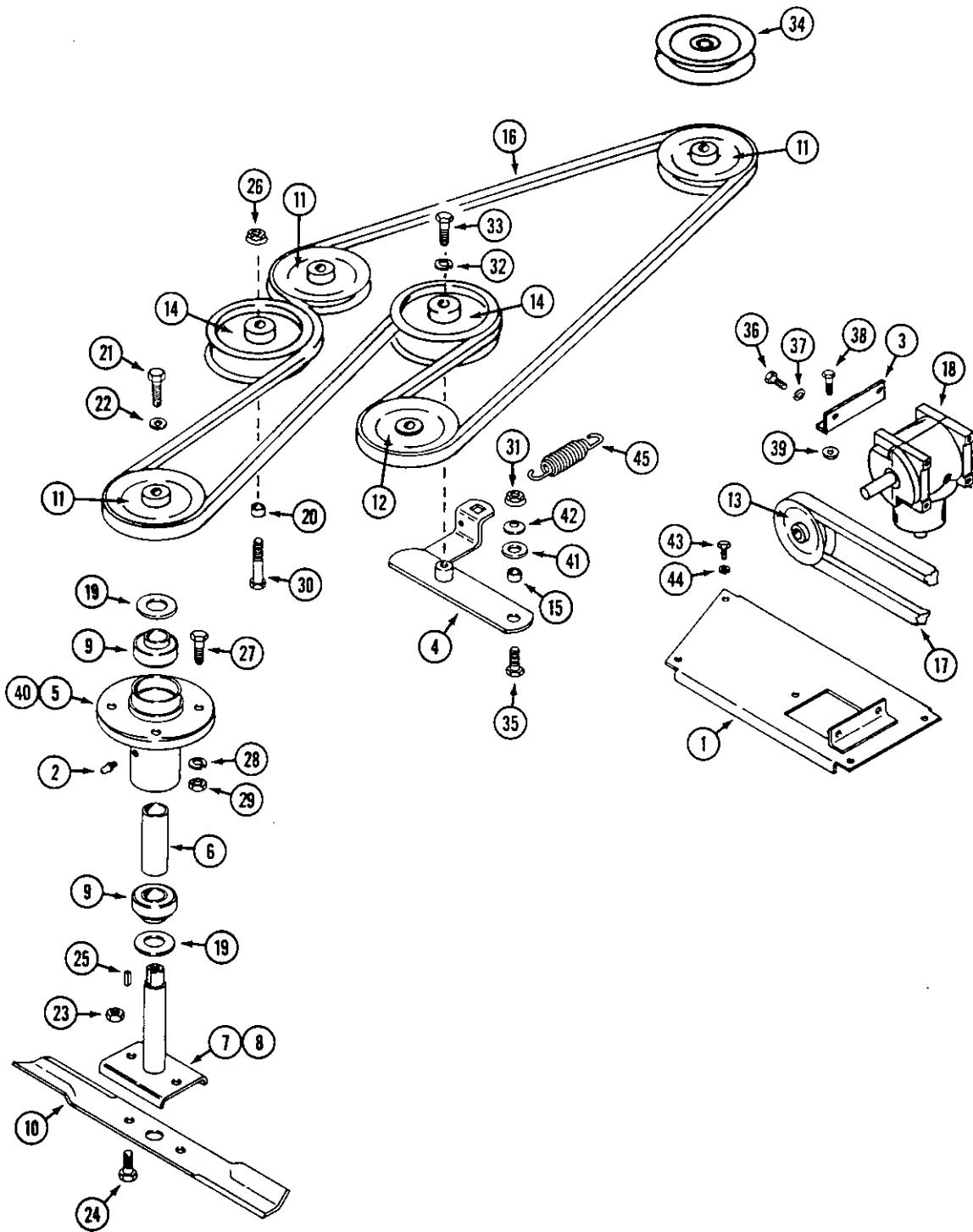
**INDEX****52SD MOWER DECK AND ATTACHING PARTS**
