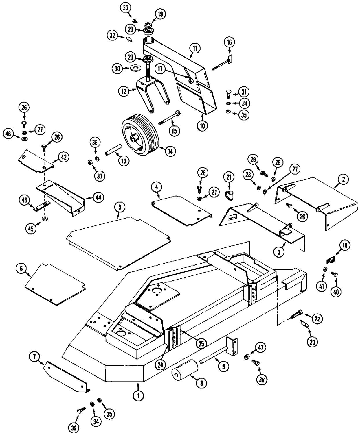
**INDEX****52SD MOWER DECK AND ATTACHING PARTS**
