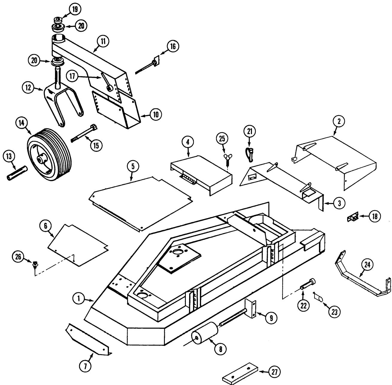
**INDEX****62" MOWER DECK AND ATTACHING PARTS**
