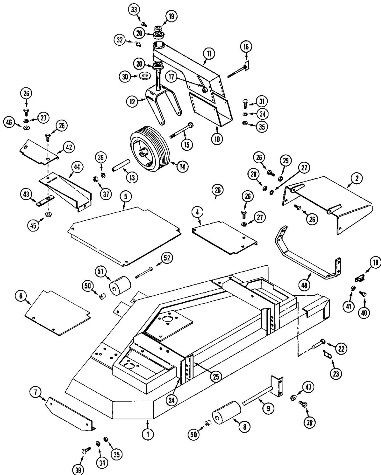
**INDEX****72" MOWER DECK AND ATTACHING PARTS**
