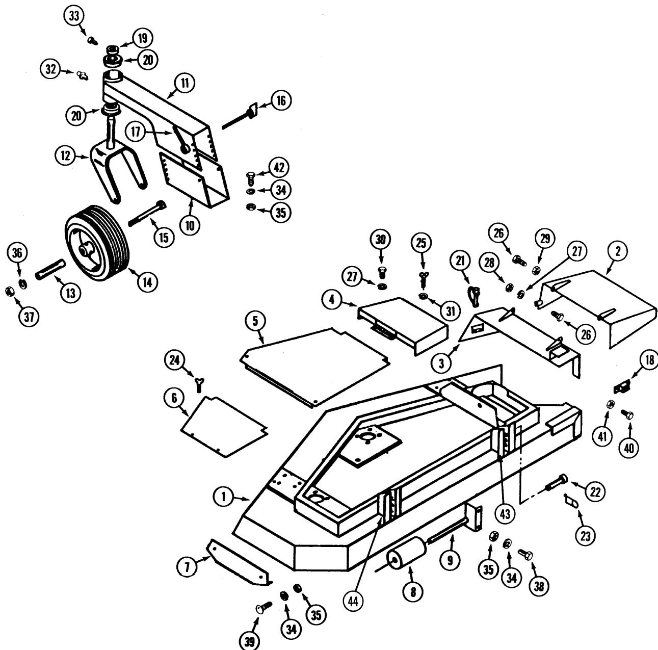
**INDEX****52" MOWER DECK AND ATTACHING PARTS**
