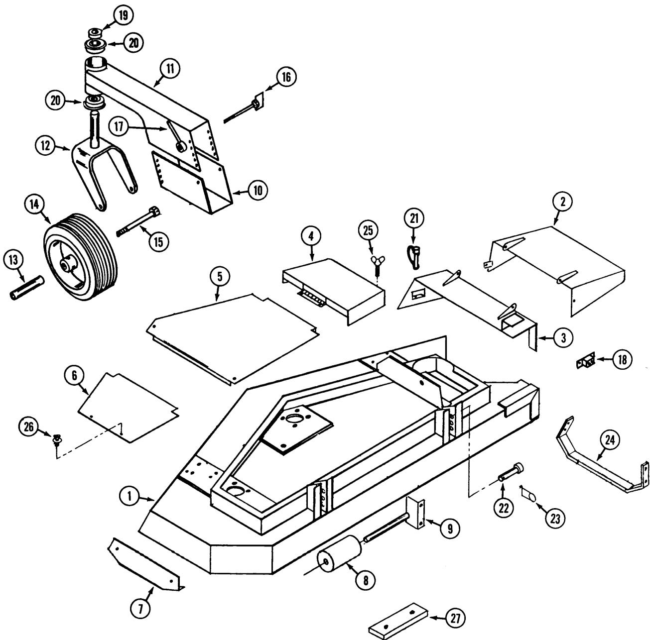
**INDEX****62" MOWER DECK AND ATTACHING PARTS**
