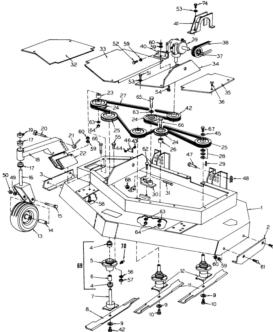
**INDEX****MOWER DECK AND ATTACHING PARTS**
