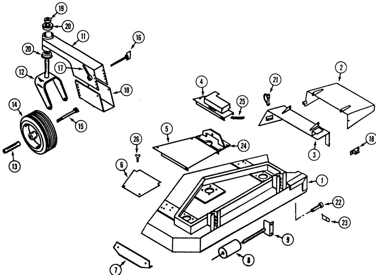
**INDEX****MODEL 42A AND 42AC MOWER DECK
