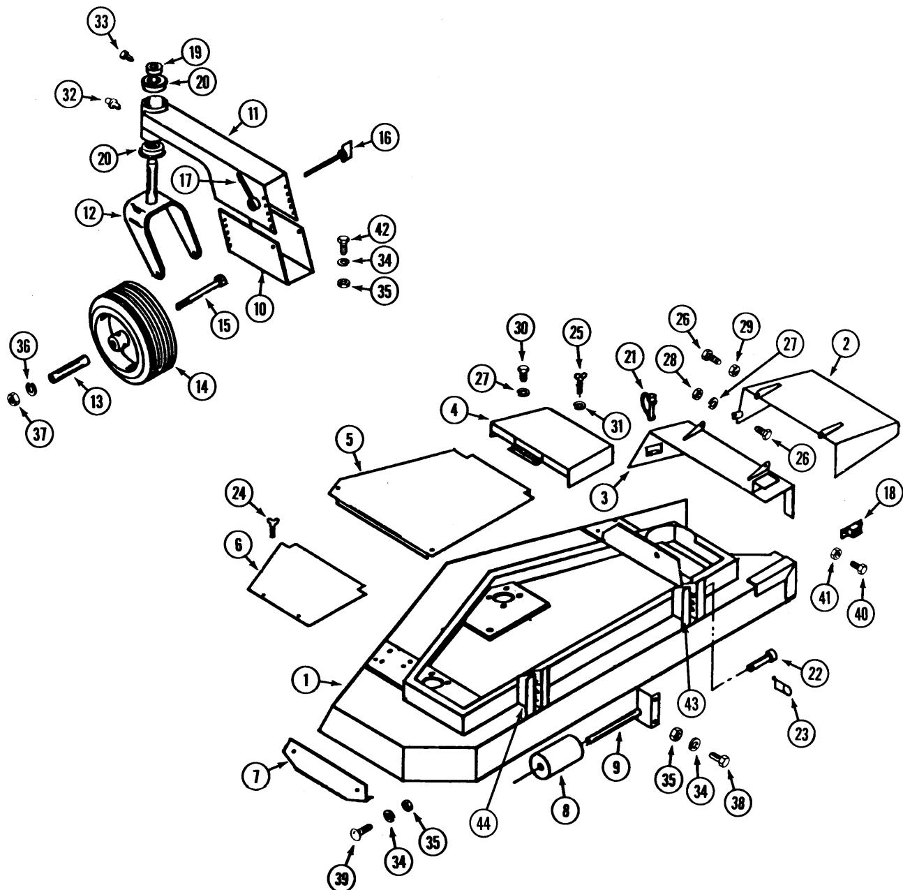
**INDEX****52" MOWER DECK AND ATTACHING PARTS**
